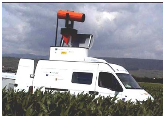
Fig. 5. The truck-based FLIDAR imaging system described by Sowinska et al. (1999)
