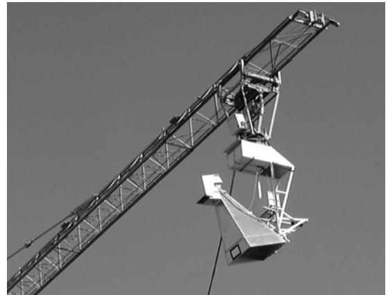
Figure 6: Polarimetric L-band TUD radiometer at INRA-Avignon-2001 experiment. The set up is mounted on a crane boom, moving over several fields, and allowed changes in azimuth and incidence angle
