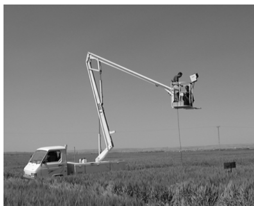
Figure 4.- Mobile equipment of the VALENCIA Anchor Station . Left hand side: mobile radiation and meteorological station. Right hand side: Truck with a 15 m boom for reflectance measurements
