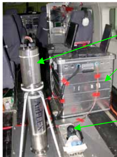
Figure 2. The Airflex sensor fixed on the floor of the CESSNA Grand Caravan airplane of the DLR. During data acquisition a video camera records the images of the context.
