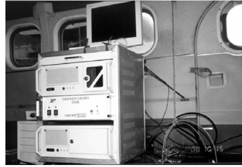
Figure 4. Airborne multiangular TIR/VNIR imaging system (AMTIS)
