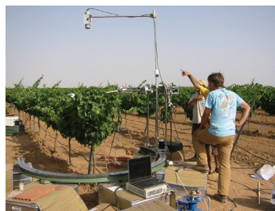
Fig. 4. Goniometer raised by 50 cm to study detail of vines (Barrax, Spain). The rotating arm is in vertical position
