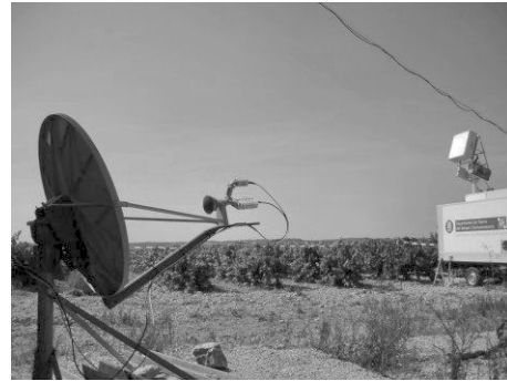
Figure 4. LAURA radiometer (right) and the antenna for the satellite connexion to the Internet (left), during REFLEX 2006, Valencia, Spain.
