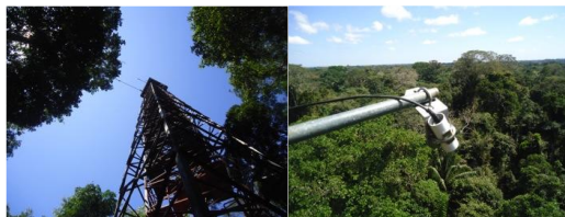
Figure 3. Pictures of the Tambopata's tower and the thermal radiometer.
