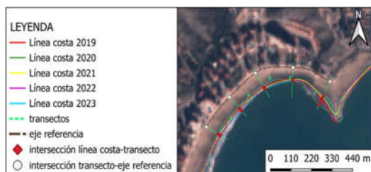
Figure 6. Extraction of the beach width through the intersection between the stretches and the coastlines of the different years (2019-2020-2021-2022-2023). Base image for 2019.
