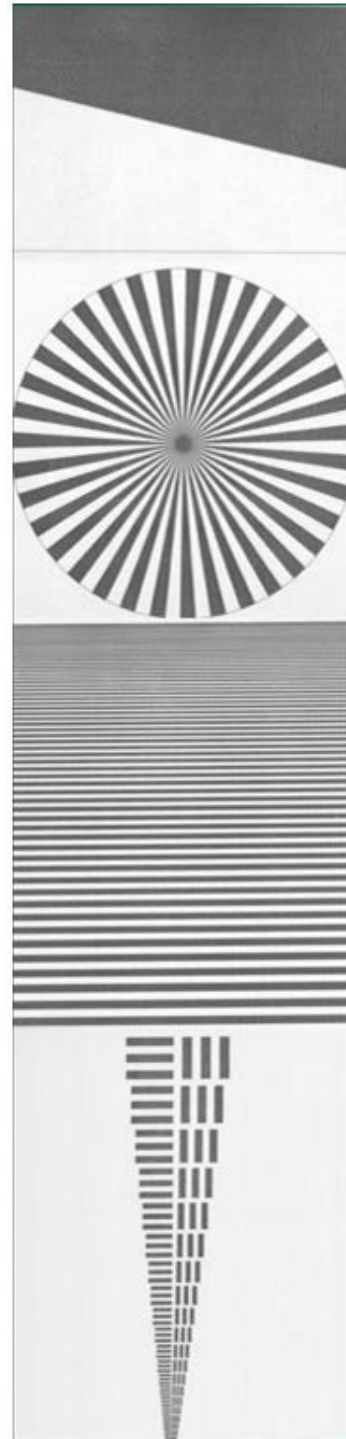
Fig. 2. Especially designed calibration field: slanted edge test, Siemens star test and two bar targets
