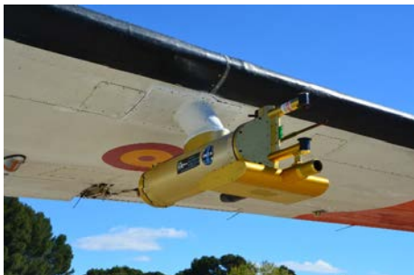
Figure 3. Probe PCAPS mounted under the left wing of the C212 s/n 30 airplane.
