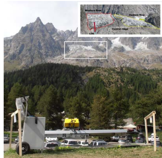
Fig. 1: GB-SAR installation. In the small rectangle a description of the two main sectors of the glacier flow, with indicated the radar LOS. In red the western side mainly moving along the LOS; in yellow the eastern one whose motion is along the yellow arrow.
